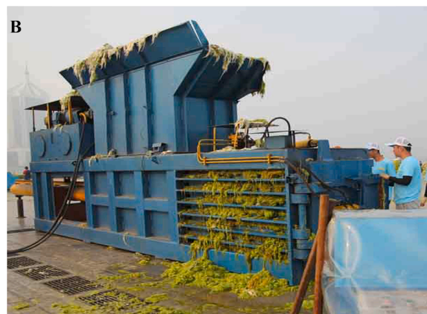
Fig. 2. Concept of electro-osmotic dewatering (EOD, A), and on-site mechanical dewatering of seaweeds at Qingdao, Shandong Province, east coast of China (B).
