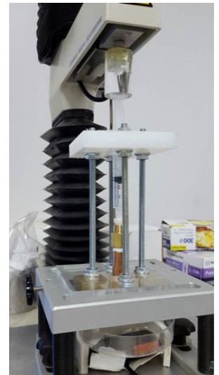
Figure 11. Fully constructed assembly. Texture Analyzer is capable of compressing syringe at a stable 1 mm/s.
