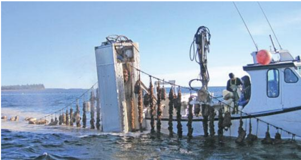
Figure 34. Innovative water pressure system funded by DFO to solve tunicate fouling problem on PEI
