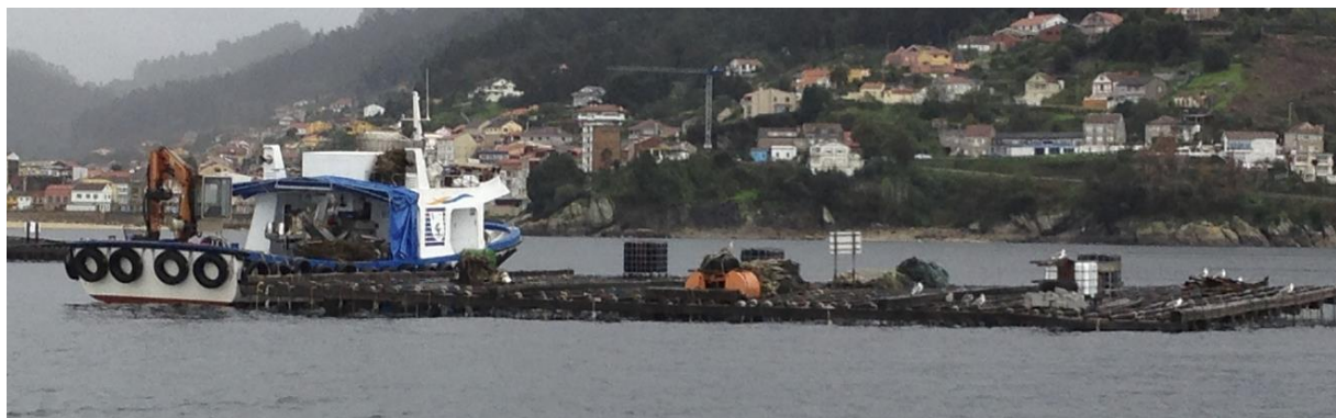
Figure 24. A mussel harvest vessel next to a 20 x 27 m mussel raft in Ria Muros
