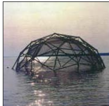
6. Trident Cage circa 1992. Geodesic design, submersible but with interior single unit net. No longer made or in use.
