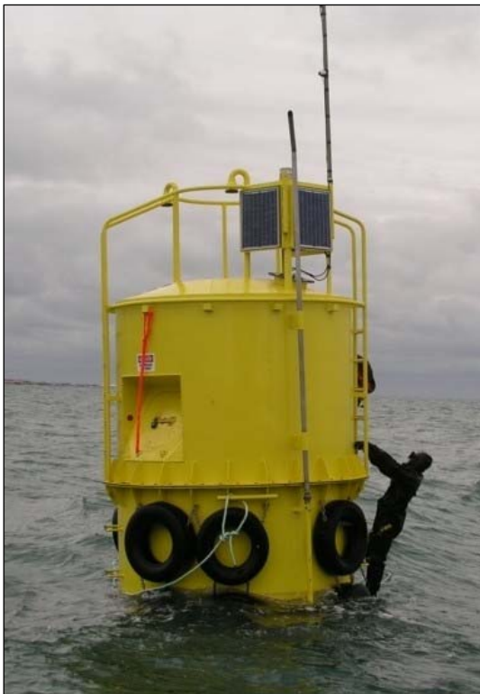
Figure 3.1. Prototype offshore fish feeder and drawing of 20-ton commercial design.
