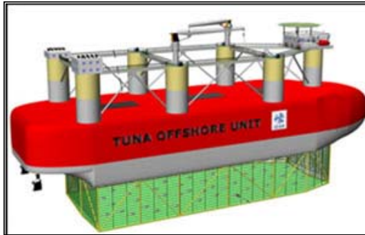
13. Ocean going concept cage , Spain, circa 2004. Specially designed for tuna where wild caught juveniles are used
