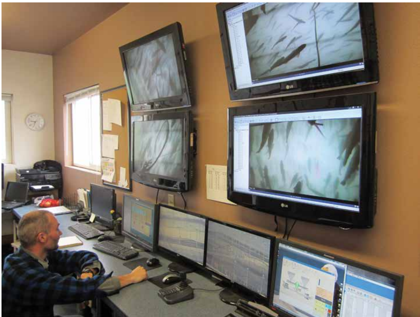
Figure 3. Control room for a salmon farm in Washington State. Fish feeding, behavior, and health are monitored using underwater video and water quality data are collected and displayed on computer screens. Feeding is done based on a computer-controlled system, feedback from the video, and the operator's experience. Photo by Laura Hoberecht.
