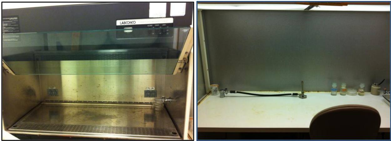
Figure 13. Two types of clean hoods. Left, a biological safety cabinet, suitable for working with cultures or hazardous materials. Right, a laminar flow cabinet, suitable for working with cultures and non-hazardous materials.
