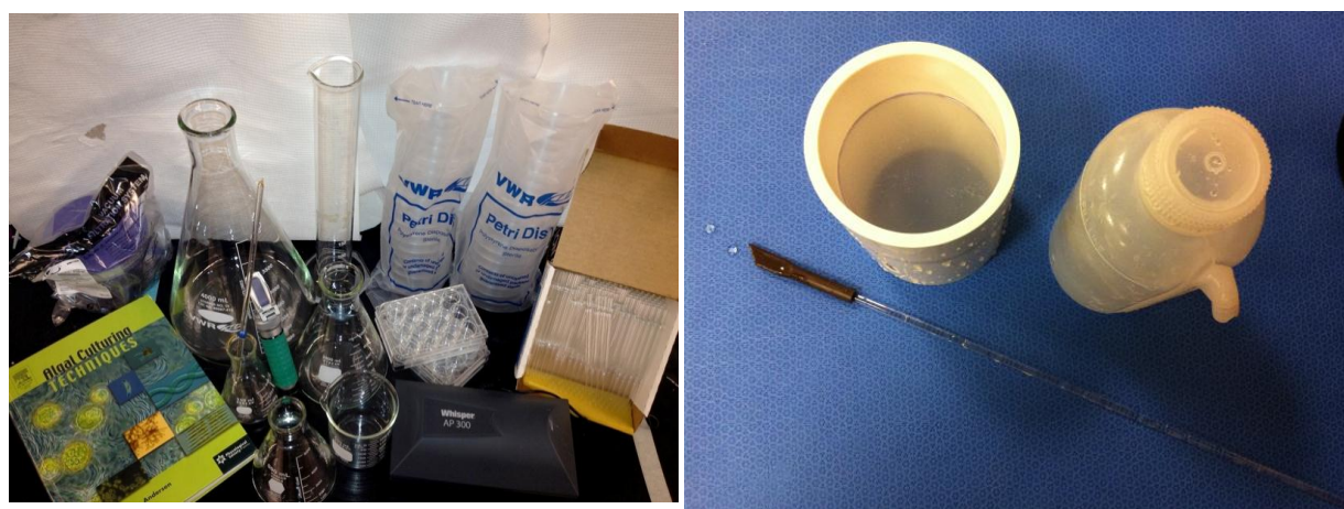
Figure 12. Necessary laboratory equipment for successful cultivation: Left: sterile vacuum filter for making stock solutions, “Algal Culturing Techniques”, various sized Erlenmeyer flasks, beaker, refractometer, thermometer, graduated cylinder, Petri dishes, multiwall plates, air pump, and Pasteur pipettes. Right: Custom filter (10-100 micron mesh), squirt bottle with sterilized seawater, and glass stir rod with rubber policeman scraper useful for
