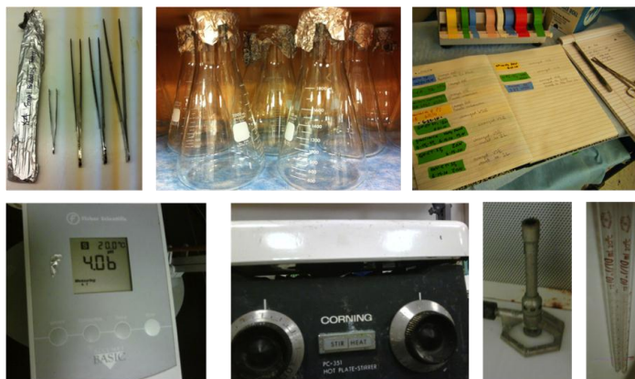
Figure 11. Useful lab items (from top left to right): forceps, sterilized glassware, lab book, pH meter, stir plate, Bunsen burner, pipettes.
