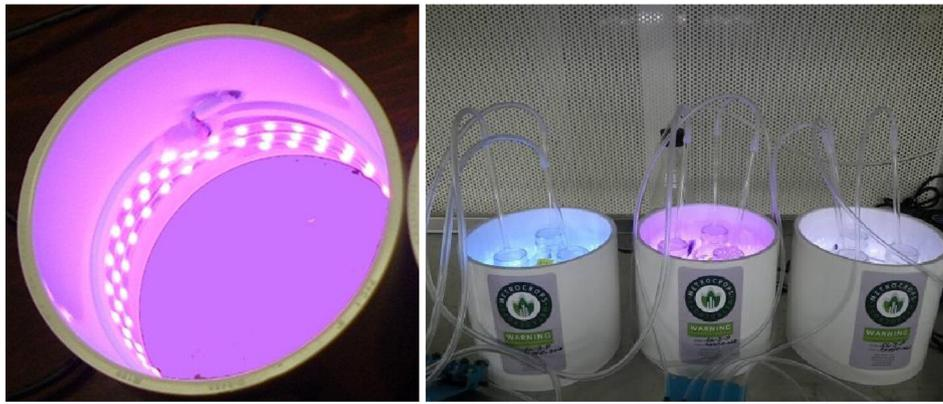
**Fig. 1.** Photographs of LED illumination cylinder. A *Gracilaria* cultivation system from the trichromatic experiment (right). A PVC tube has three 0.5 m circles of LED strips inside. Each white “square” in the tube is an LED package. Each package contains one red chip, one blue chip, and one green chip (left). From right to left: RGB, RgB and rGB.
