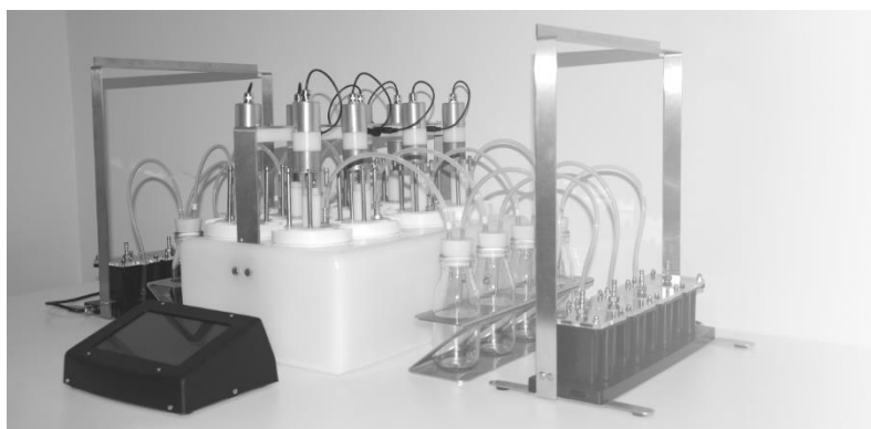
Figure 1. CJC biomethane potential system (courtesy of CJC labs).
