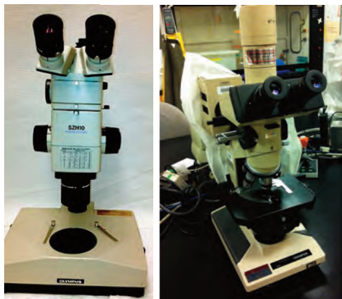
Figure 2-8. Dissecting (left) and compound (right) microscope.
