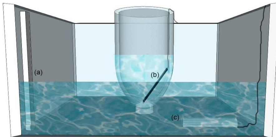
**Figure 14** – 3D representation of the system used to hatch the *Artemia* cysts. (a) Represent the thermometer used to control water temperature; (b) is the aeration probe inside the bottle where the cysts are hatched; (c) is the thermostat used to keep the water temperature stable.
