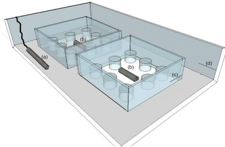
**Figure 12** – 3D representation of one of the two boxes of the system for larvae bioassays. (a) Thermostat to keep the water temperature stable; (b) iron bars were put in the small boxes to avoid the fluctuation; (c) and (d) indicate the water level used to conduct the temperature of the small boxes and the exterior box, respectively. Each box contained 8 cups for putting the mosquito larvae.
