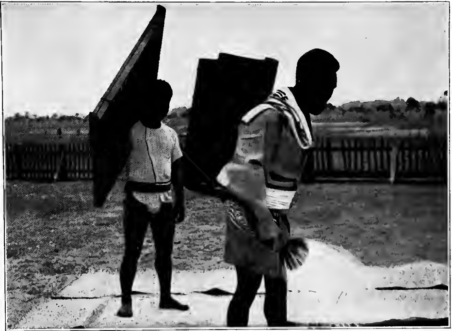
SPRINKLING THE SHEETS TO PREVENT CURLING.
