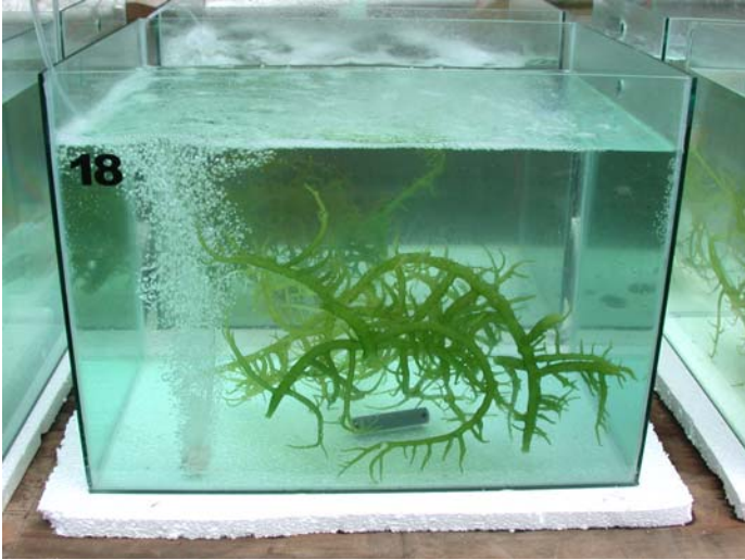
Figure 6: Glass aquarium tank used to hold the seaweed; contains air stone and a temperature logger (grey cylindrical).
