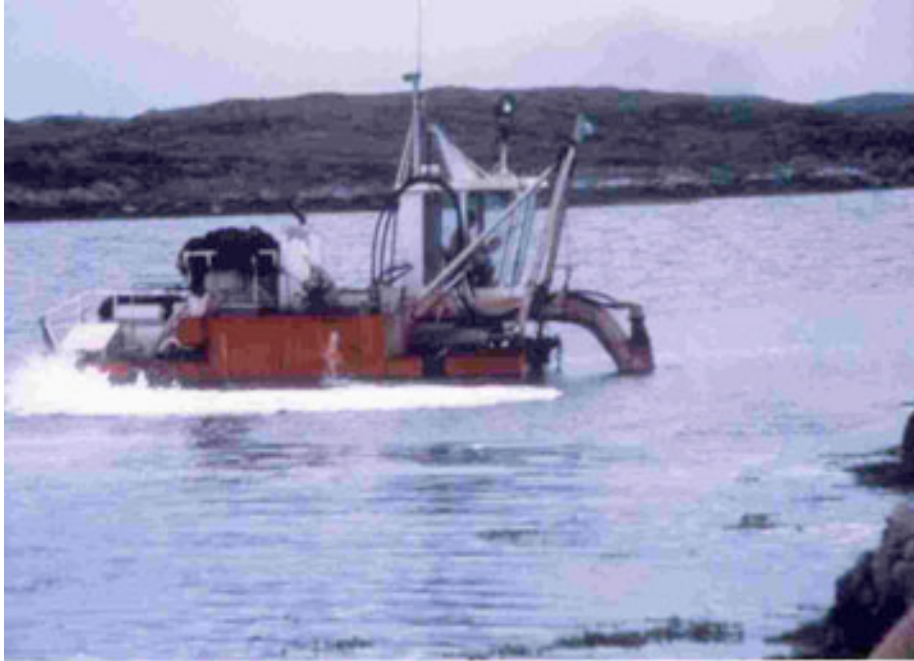
Fig.12: Harvesting of Ascophyllum nodosum with a Norwegian suction cutter from Pronova Biopolymers Ltd. in southwest NS. (photography by J. Pringle).
