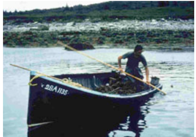
Fig. 7: Harvesting of Chondrus crispus by a “wincher” boat off Cape Gage, PEI. The crew is bringing three rakes, attached together, on board while three others are dragged on the other side.
