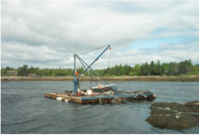
Fig. 20: Alternative methods of unloading the daily Ascophyllum nodosum harvest in floating devices (platforms) in areas of southern NB where access to wharfs is difficult.
